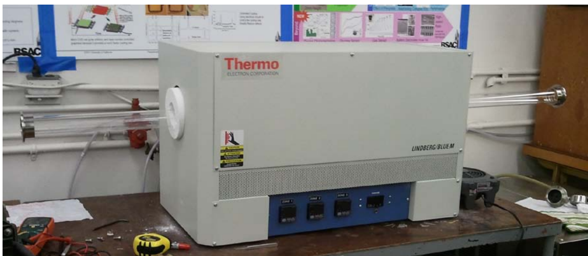
Figure A.4. Thermal furnace loaded with a 2-inch quartz tube. The fan on the right side of the furnace is used to cool the 720°C tube into a temperature below 200°C within 10min.
