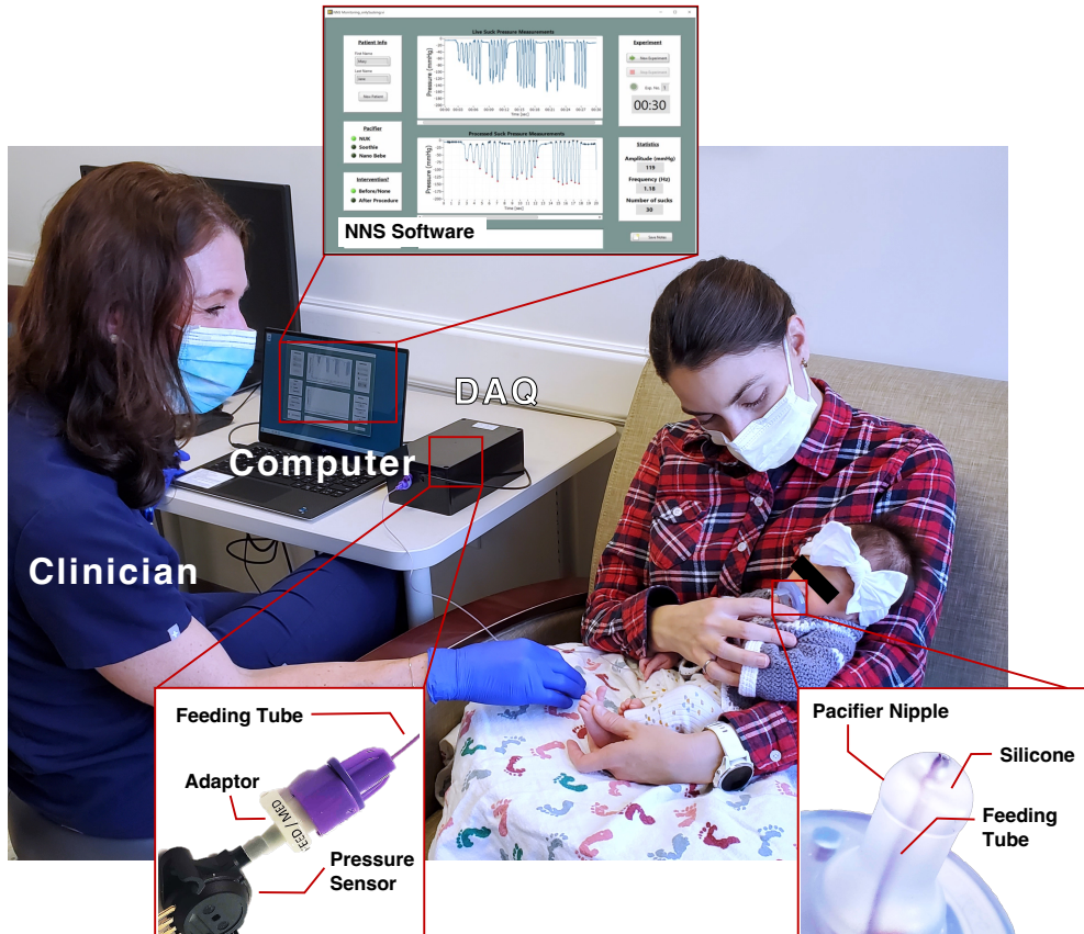
Figure 3.1: An image of the non-nutritive suckling measurement system to measure intraoral vacuum profiles of infants. The system is comprised of an instrumented pacifier, pressure sensor, data acquisition board (DAQ), and computer.
