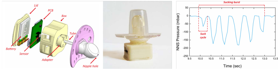
Figure 1.17: Compact NNS measurement system devised by Ebrahimi et al. [15].
