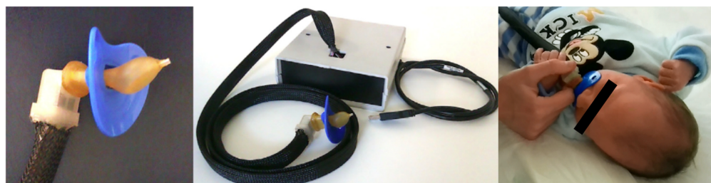
Figure 1.14: Sensorized pacifier system proposed by Grassi et al. [13].
