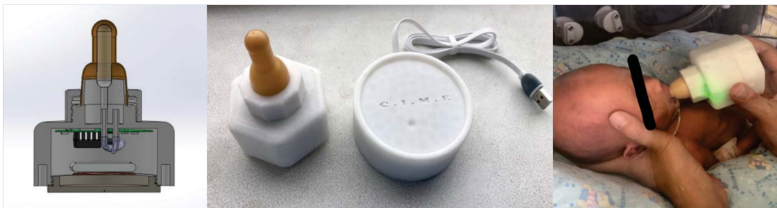
Figure 1.16: Compact pacifier NNS measurement system proposed by Akbarzadeh et al. [14].
