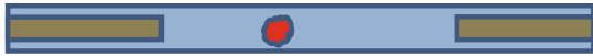
Fig. 1 Cartoon representation of an idealized cryo-EM specimen. Note that the particle ( red ), the hole in the carbon film ( brown ), and the thin film of vitreous ice ( blue ) are not drawn to scale. The main point of this cartoon is to illustrate the goal that the particle should be surrounded on all sides by vitrified buffer, and—in particular—the particle should not touch the air–water interface
