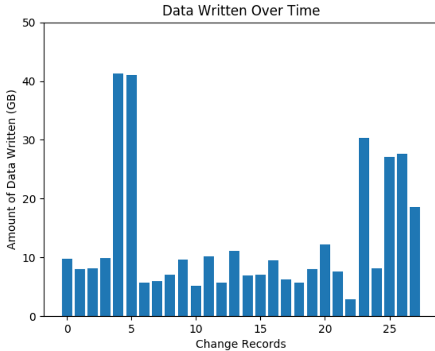
Figure 6.7: Amount of data written to the SSD between each pair of snapshots.
