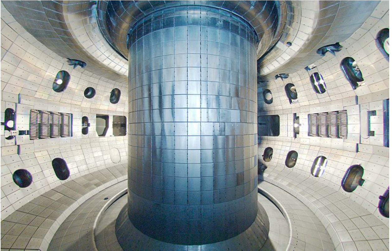
Figure 1.2: The inside of the DIII-D tokamak [2]. Note the center-stack, various diagnostic and neutral beam ports, and the RF antennas. The walls are graphite.
