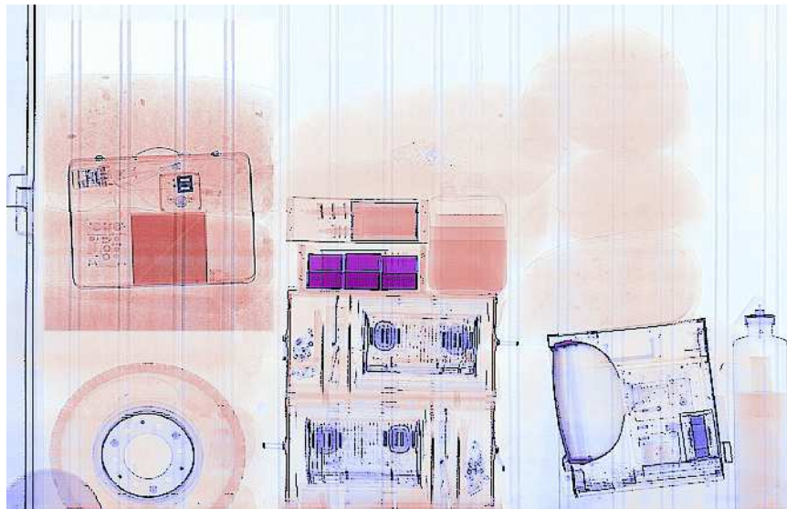
Figure 4.1 The visualization of system proposed by Ogorodnikov and Petrunin. Image of container in TZ-palette: organic–red, inorganic–blue, heavy metals–lilac. (Image obtained from [6])
