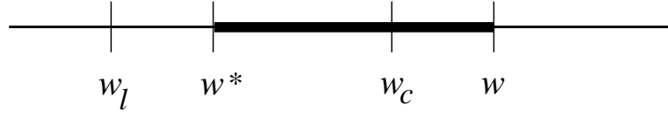
Figure II.1: Relationship between various wirelength quantities. w is a placer’s suboptimal wirelength result. w^* is the optimal result. w_l is a lower bound. w_c is a pre-calculated wirelength. w - w^* is the suboptimality gap.
