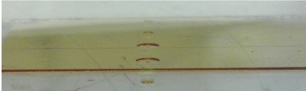
Figure 4.9: Test pattern of AZ 125 nXT on a glass slide used to demonstrate 300 \mu\text{m} thick photoresist process.
