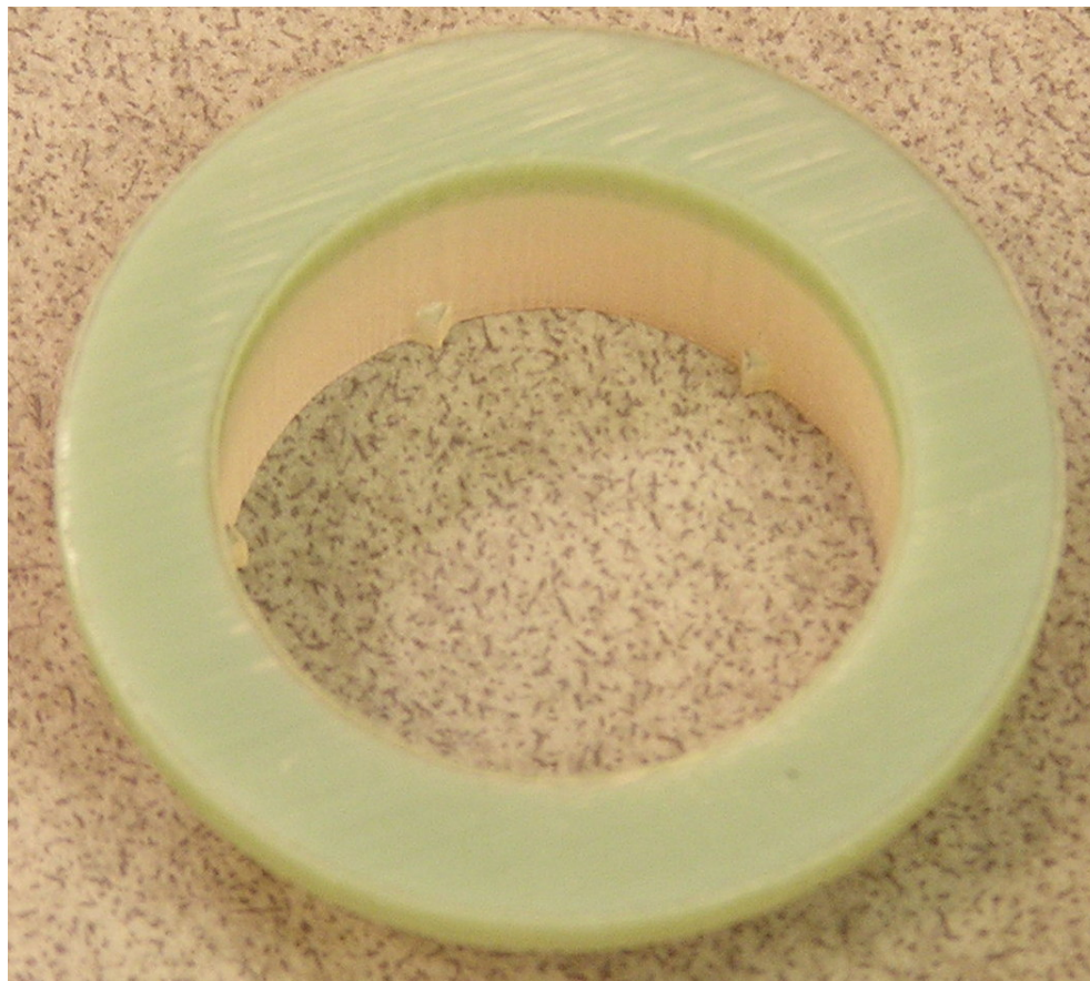
Figure A.1: A picture of the 3D printed ring designed to keep the salt pill from making conductive contact with the magnet wall.
