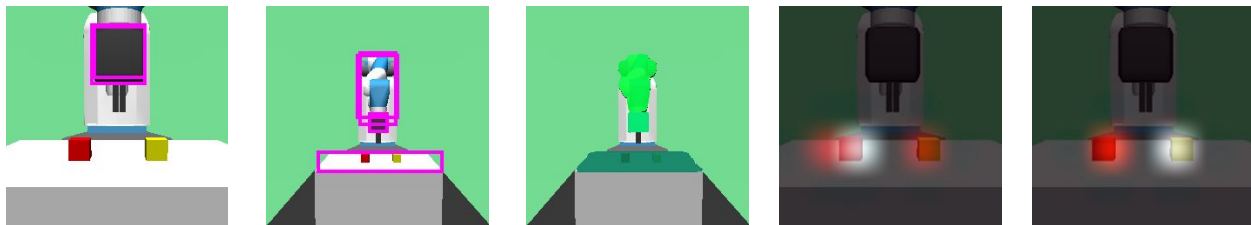
Figure 4.3: a) Mask R-CNN object detection results b) Mask R-CNN detection results on far view c) Mask R-CNN instance segmentation results on far view d) Grad-CAM result with 'red block' text input (white being highest intensity) e) Grad-CAM result with 'yellow block' text input (white being highest intensity).
