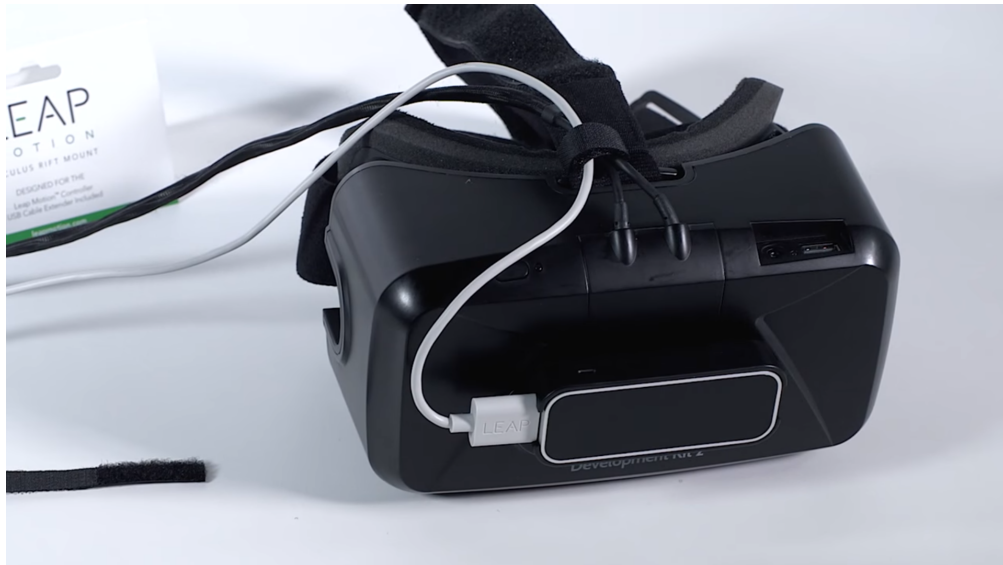
Image 3.1: The Oculus Rift DK2 headset with the LEAP Motion Controller attached. [Mot17b]
