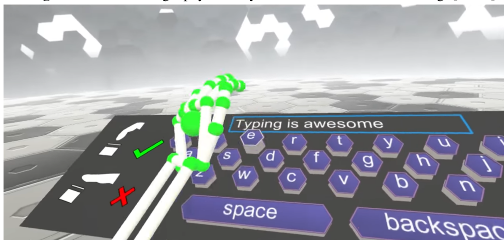
Image 2.2: A demo with a 3D keyboard and hand motion tracking where the user must press down each key. [Cor16]
