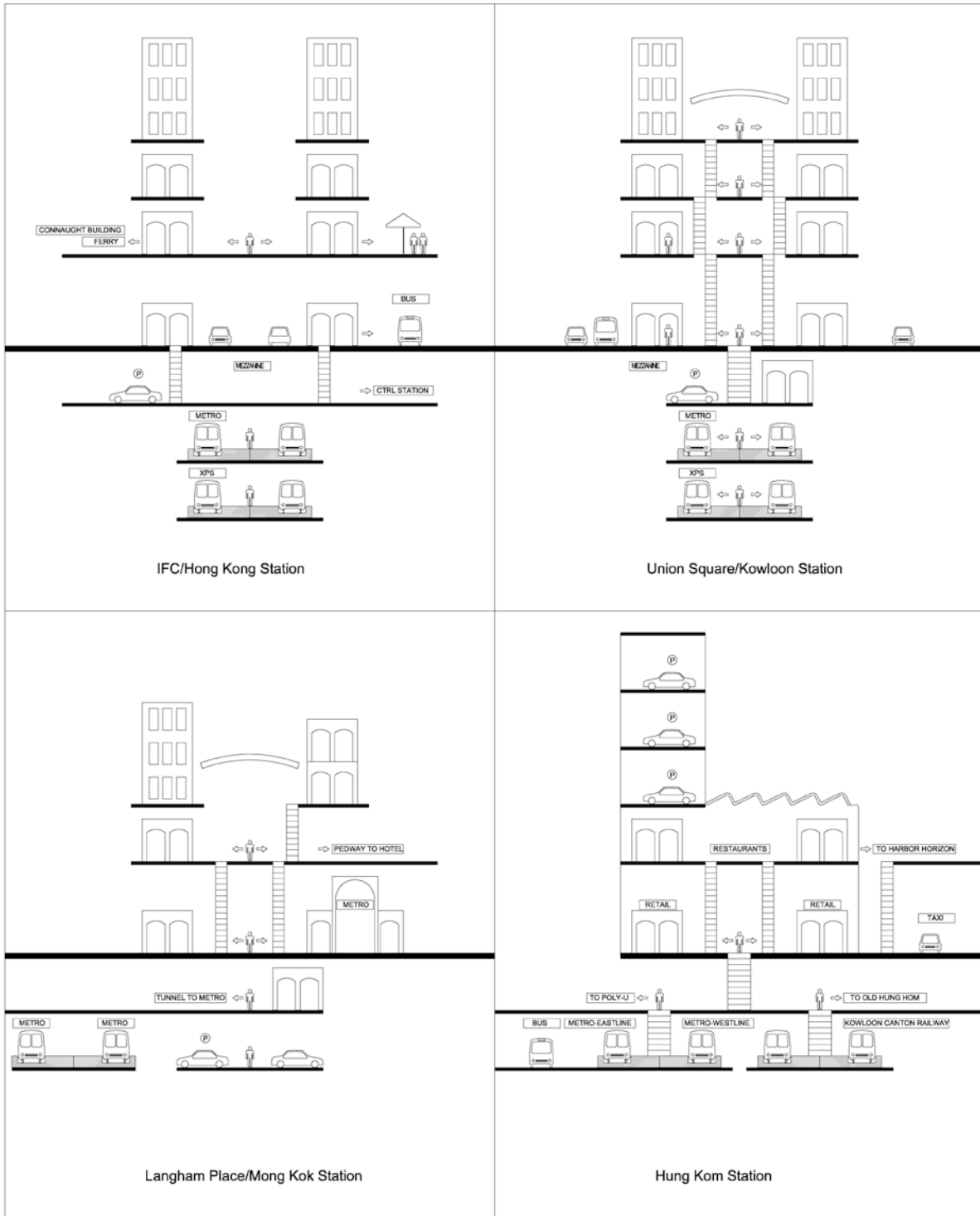
Figure 17. Author's diagram comparing the sectional organization of: (1) Hong Kong Station and IFC complex; (2) Union Square, Kowloon Station; (3) Langham Place, Hong Kong; and (4) Hung Hom Station. It shows how infrastructure, retail, towers, motorways, and bus terminus are vertically integrated.
