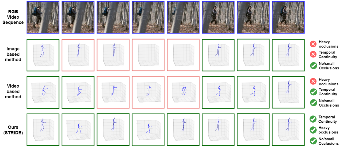
Figure 1.1: Effect of occlusions on pose estimation. Image-based 3D pose estimators [4] often struggle with heavy occlusions, as illustrated in this figure. Without temporal context, predictions on highly obscured frames are inconsistent with prior poses, like the erroneous pose in the third frame. Notably, even state-of-the-art video approaches [63] fail on prolonged full occlusions spanning multiple frames, as in frames 4-5. This highlights another critical limitation - models are brittle when deployed outside their training distributions. Without training examples of such long-duration occlusions, models fail to extrapolate reasonable poses. Our work addresses this through test-time training of a human motion prior. By fine-tuning on each new video, we tailor this parametric prior to handling sequence-specific occlusion patterns not observed during training. Given an initial noisy estimate, our approach refines the pose sequence into an accurate, temporally coherent output, as shown in the final row.
