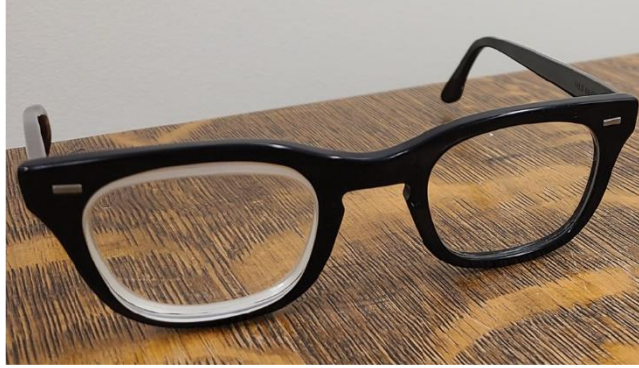
Figure 2.2 Experimental spectacles with a horizontal magnifier over the right eye.
