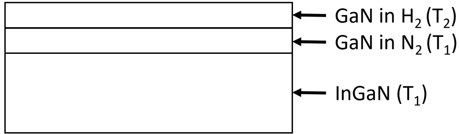
Figure 3.10: General layer structure of a single period of strain-relaxed InGaN buffer with smooth surface morphologies without the presence of v-pits. These changes of increased temperature in interlayers, lower V/III ratio and inclusion of hydrogen all work to increase adatom mobility and lateral diffusion across the surface, allowing the growth to fill in voids and pits.
