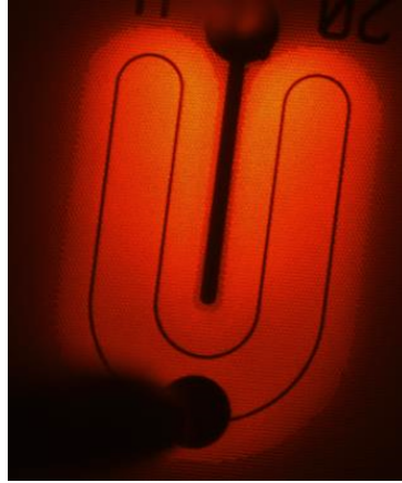
Figure 4.5: Photograph of device under operation at 50 \text{ A cm}^{-2} .
