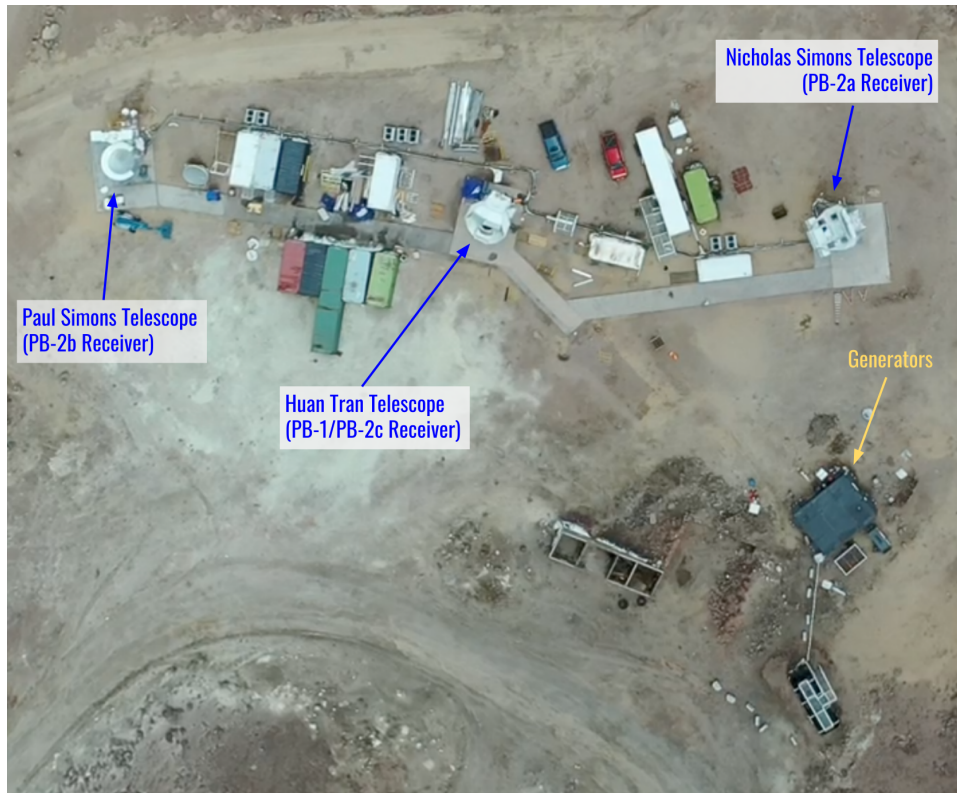
Figure 2.13: Aerial view of the SA site. The telescopes roughly form a line in the north-south direction, with the Nicholas Simons Telescope (PB-2a receiver) on the north end, the Paul Simons Telescope (PB-2b receiver) on the south end, and the Huan Tran Telescope (originally PB-1 receiver, planned PB-2c receiver) in the center. The structure that houses the site generators is shown in the bottom right corner of the photo. Also seen in the image are the various shipping containers that house the telescope control electronics and computers, compressors for the receiver cryogenic systems, and general storage items. Photo thanks to Nolberto Oyarce.
