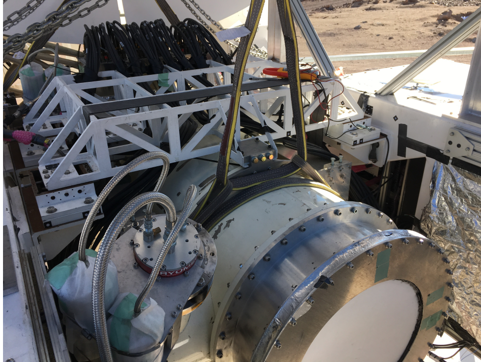
Figure 2.10: Photo of the PB-2a receiver mount installed on the Nicholas Simons Telescope from 2019. The rigging equipment seen in this photo is from installation of these parts and is not present while the telescope is operating. The steel truss structure and three of its four attachment points to the telescope can be seen, along with the front attachment point between the receiver and the truss. Hinges that are obscured in this view of the telescope connect the rear part of the truss structure to the receiver via I-beams along the receiver sides.
