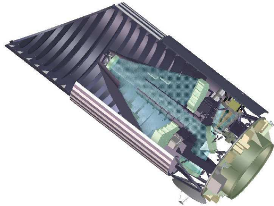
Fig. 11.— Cutaway view of the reference SNAP design. The entire telescope attaches to the spacecraft structure by means of bipods. The outer baffle, shown cut away, also attaches to the spacecraft structure by means of its separate supporting struts. A discardable door, shown open in light gray, protects the cleanliness of the optics until on-orbit commissioning begins. Solar panels are fixed, not deployed.
