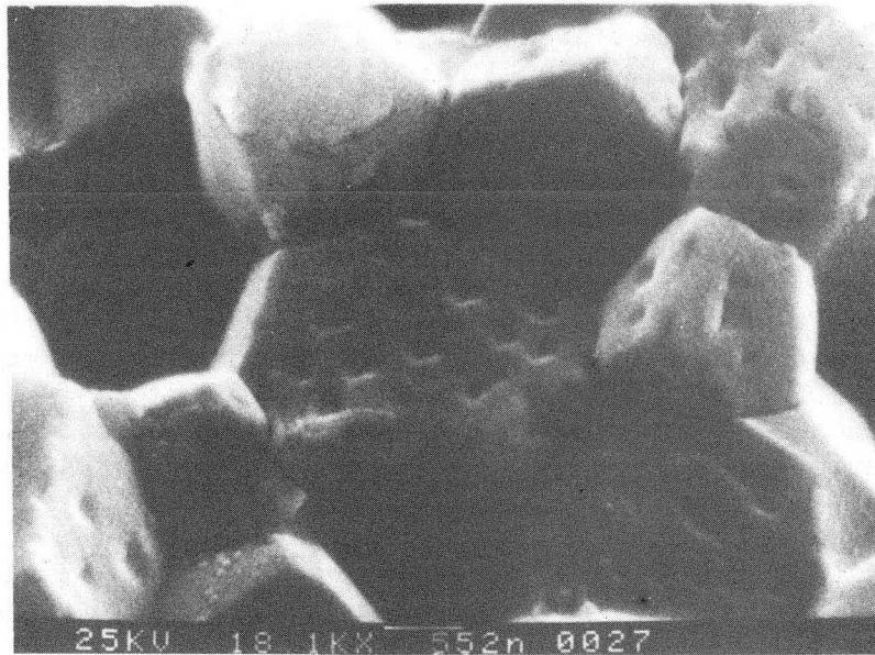
Fig. 6. a) A schematic of crack growth characteristics for extrinsic cracks indicating the threshold, K_{th} , the critical stress intensity, K_c , and the intervening region of creep crack growth. b) A scanning electron micrograph of a growing crack profile, indicating coplanar damage. c) A scanning electron micrograph of a crack growth surface revealed by brittle fracture at room temperature, showing cavities on two grain interfaces.
