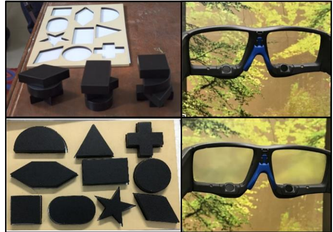
Figure 1. Materials. Left: The Seguin Form Board Test (SFBT). Top: before. Bottom: after. Right: Blurring method. Top: no blur. Bottom: intermediate blur level.
