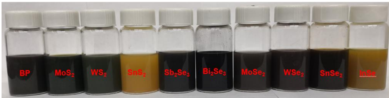
Figure 4.7 A total library of nanosheet inks produced from in lab grown crystals that were exfoliated through top-down electrochemical intercalation of large ammoniums and exfoliation.
