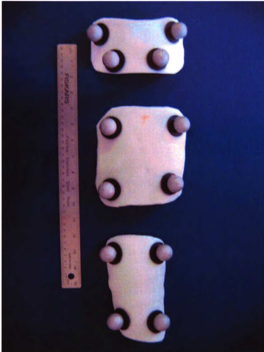
Figure 6: (From Top to Bottom) Hip Marker Cluster, Thigh Marker Cluster, Shank Marker Cluster
