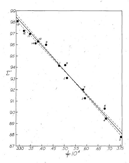
Fig. 3. \(\Sigma''\)-versus-l/T plot from the data of Table I. The points are numbered in the order in which they were measured. The solid line is the best straight line that could be drawn through the points by eye. The dashed lines show the limits of uncertainty in the slope of the line.
