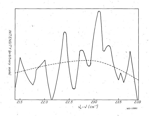
Fig. 9. Infinitely resolved profile of Swan (0-0) band head (solid line). Dotted line represents profile of instrumental recording.  $\nu_0$  is frequency of origin of band in cm<sup>-1</sup>.
