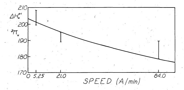
Fig. 5. Heat of formation at 0°K of the <sup>3</sup>II state of C<sub>2</sub> determined at three different scanning speeds. The heights of the points represent the uncertainties in the heats. The correct heat corresponds to the intersection of this curve with the ordinate.
