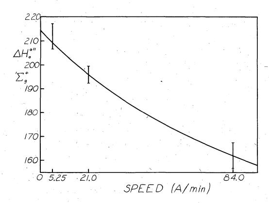
Fig. 6. Heat of formation at  $0^{\circ}$ K of the  $^{1}\Sigma_{g}^{+}$  state of  $C_{2}$  determined at three different scanning speeds. The heights of the points represent the uncertainties in the heats. The correct heat corresponds to the interception of this curve with the ordinate.
