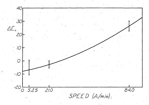
Fig. 7. Difference in energy between the  ${}^3\Pi_u$  and the  ${}^1\Sigma^+_g$  states of  $C_2$  determined at three different scanning speeds. The heights of the points represent the uncertainties in the heats. The correct energy difference corresponds to the interception of this curve with the ordinate. A negative value for this quantity means that the  ${}^3\Pi_u$  state is lower than the  ${}^1\Sigma^+_g$  state.
