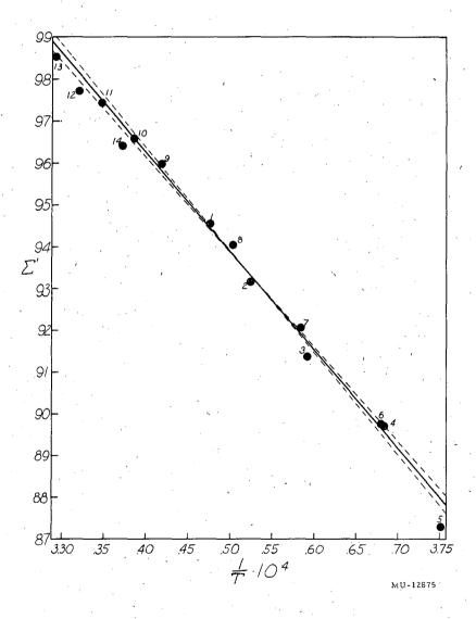
Fig. 2. \( \subseteq \text{-versus-l/T} \) plot from the data of Table I. The points are numbered in the order in which they were measured. The solid line is the best straight line that could be drawn through the points by eye. The dashed lines show the limits of uncertainty in the slope of the line.
