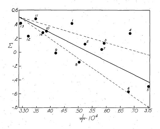
Fig. 4. \(\Sigma\)-versus-l/T plot from the data of Table I. The points are numbered in the order in which they were measured. The solid line is the best straight line that could be drawn through the points by eye. The dashed lines show the limits of uncertainty in the slope of the line.
