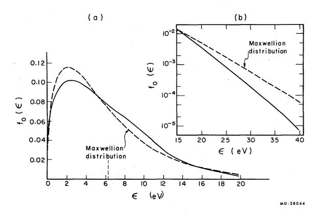
Fig. 8. The electron-energy distribution in  $H_2$  calculated with  $v_d = 1.88 \times 10^7$  cm/sec (so  $mv_d^2/2 = 0.1$  eV) and using the collision frequency for electronic excitation, shown in Fig. 2, multiplied by 4.7. The Maxwellian distribution shown has the same mean energy, which is indicated by the vertical dashed line. The inserted drawing (b) shows the "tail" of the distribution on a logarithmic scale.
