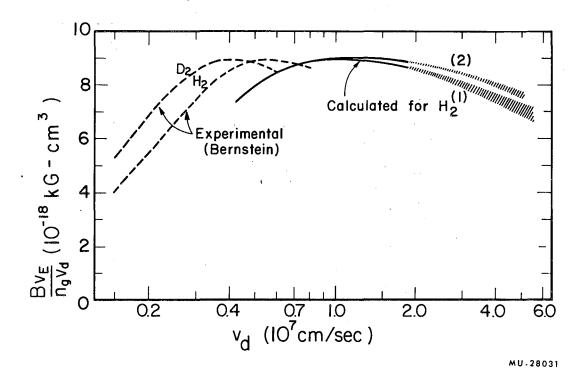
Fig. 5. The electron drift speed  $v_{\overline{E}}$  in the drift frame. The collision frequency for electronic excitation shown in Fig. 2 was multiplied by unity for curve (1) and by 4.7 for curve (2).
