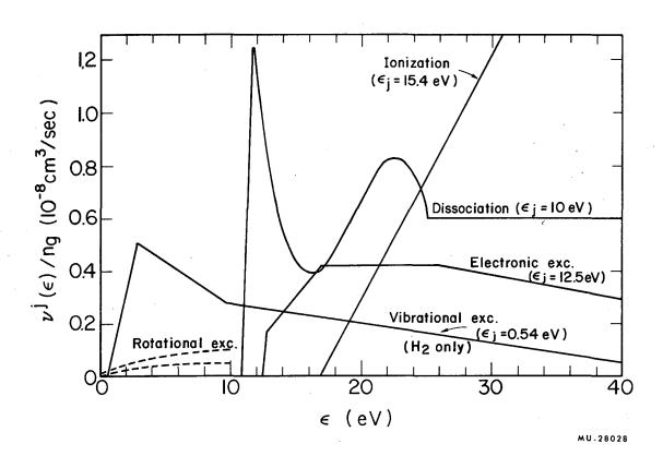
Fig. 2. Collision frequencies  $v^j$  and energy transfers  $\epsilon$  used in the numerical computations.
