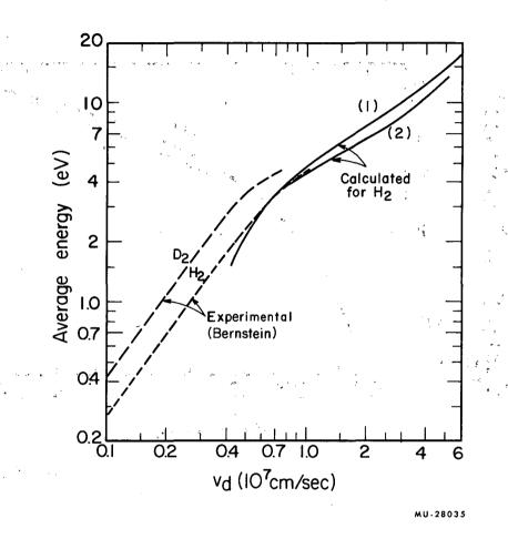
Fig. 11. The mean energy of the electrons in the gas frame. The collision frequency for electronic excitation shown in Fig. 2 was multiplied by unity for curve (1) and by 4.7 for curve (2).
