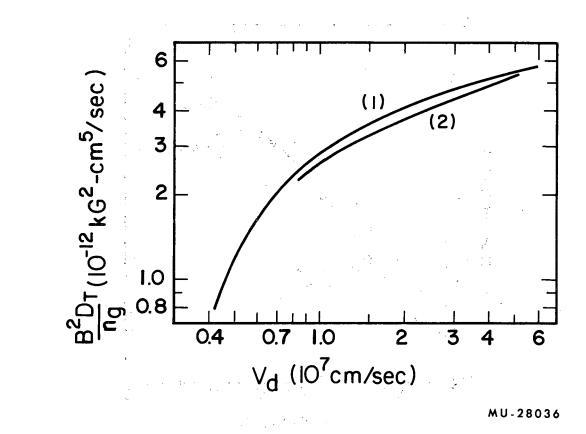
Fig. 12. The coefficient for diffusion across the magnetic field. The collision frequency for electronic excitation shown in Fig. 2 was multiplied by unity for curve (1) and by 4.7 for curve (2).
