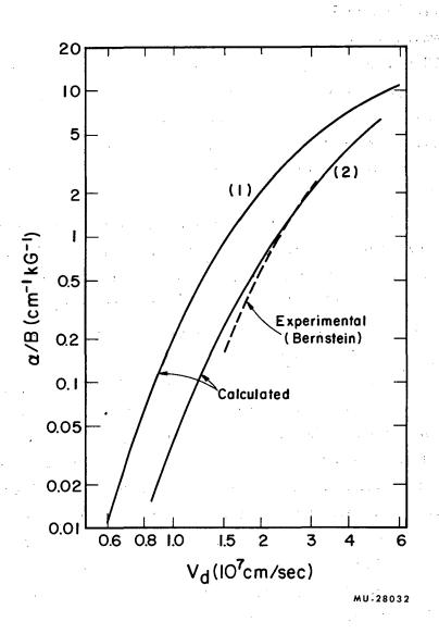
Fig. 6. The ratio of the Townsend coefficient a to the magnetic field B in H<sub>2</sub> gas. The collision frequency for electronic excitation shown in Fig. 2 was multiplied by unity for curve (1) and by 4.7 for curve (2).
