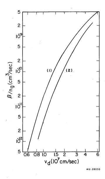
Fig. 4. Calculated values of the ionization rate  $\beta$  in  $H_2$  gas using the collision frequency for electronic excitation shown in Fig. 2 multiplied by unity for curve (1) and by 4.7 for curve (2).
