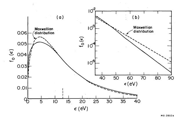
Fig. 9. The electron-energy distribution in H<sub>2</sub> calculated with  $v_d = 5.14 \times 10^7$  cm/sec (so  $m v_d^2/2 = 0.75$  eV) and using the collision frequency for electronic excitation, shown in Fig. 2, multiplied by 4.7. The Maxwellian distribution shown has the same mean energy, which is indicated by the vertical dashed line. The inserted drawing (b) shows the "tail" of the distribution on a logarithmic scale.
