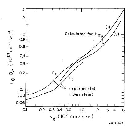
Fig. 10. The coefficient of diffusion along the magnetic field. The collision frequency for electronic excitation as shown in Fig. 2 was multiplied by unity for curve (1) and by 4.7 for curve (2).
