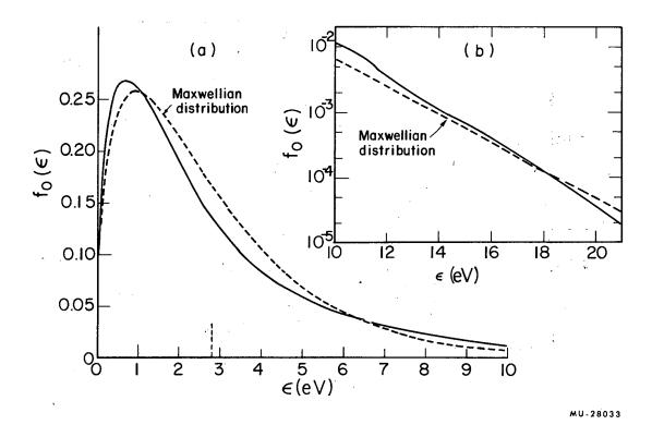
Fig. 7. The electron-energy distribution in  $H_2$  calculated with  $v_d = 5.93 \times 10^6$  cm/sec (so  $mv_d^2/2 = 0.01$  eV) and using the collision frequency for electronic excitation, shown in Fig. 2, multiplied by 4.7. The Maxwellian distribution shown has the same mean energy, which is indicated by the vertical dashed line. The inserted drawing (b) shows the "tail" of the distribution on a logarithmic scale.
