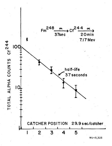
Fig. 4. Alpha recoil milking experiment.
