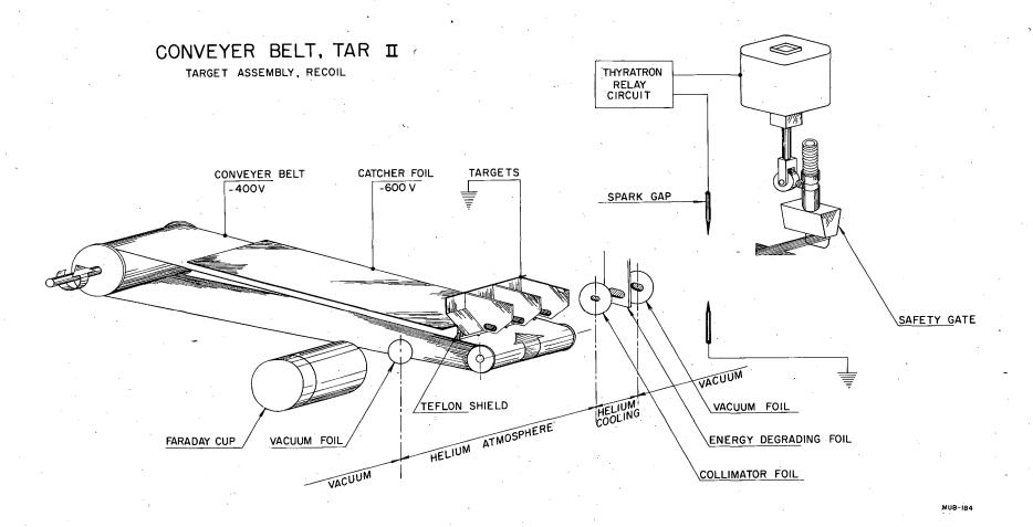
Fig. 3. Schematic diagram of conveyer belt experiment.
