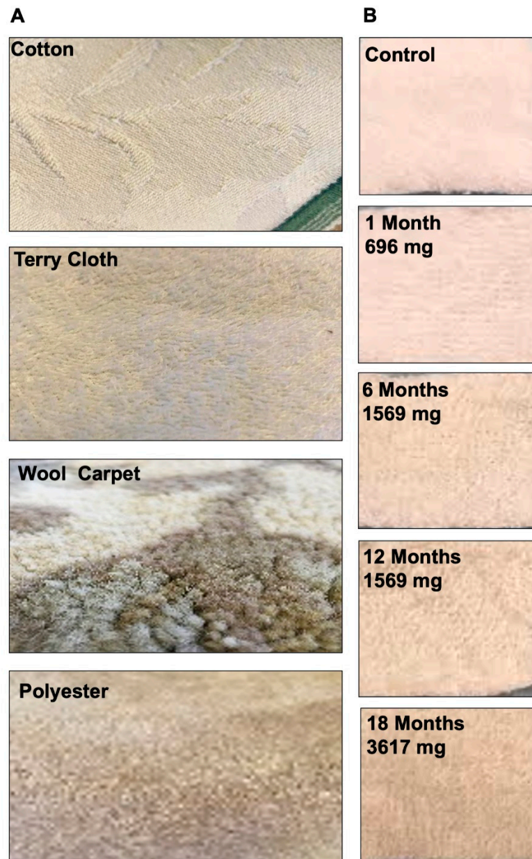
Figure 1. Common household fabrics exposed to thirdhand smoke (THS). (A) Cotton, terry cloth, wool carpet, and polyester were exposed to THS. All samples in A are unexposed fabrics. (B) Terry cloth exposed to different concentrations (mg) of particulate material from cigarette smoke at 1, 6, 12, and 18 months.
