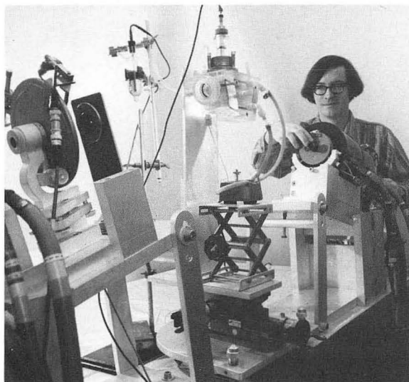
Graduate student aligns automatic ellipsometer in a boundary layer measurement.
