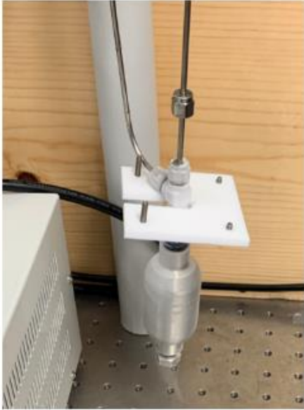
Figure 49: sample vessel is out from the cooler after procedure
