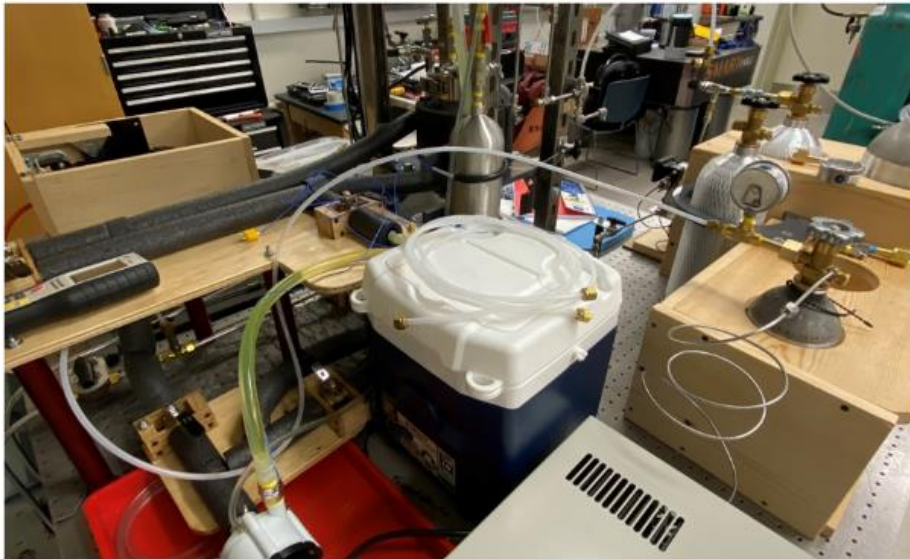
Figure 35: Sample Tank Connected to Vacuum
