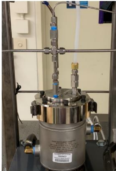
Figure 4: Pressure Vessel without Insulation
