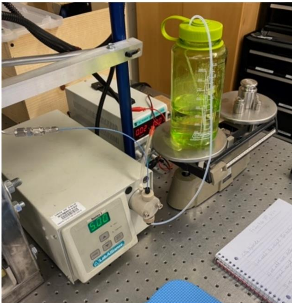
Figure 24: H 2 O Syringe Pump, Water Reservoir, and Balance with Weights for Controlling Water Input into the System
