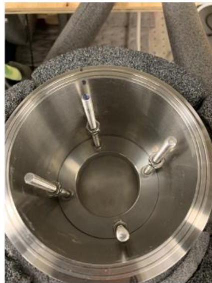
Figure 14: Installed Basket inside the vessel
