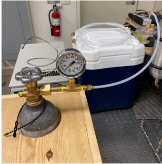
Figure 34: Sample Tank setup to Vacuum
