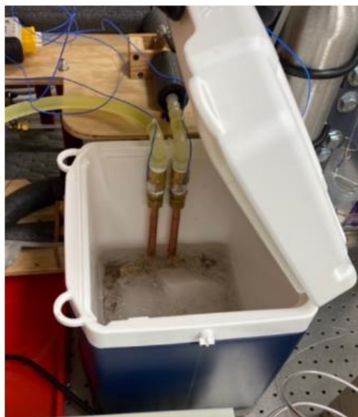
Figure 33: Auxiliary Chiller with Dry Ice
