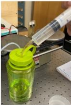
Figure 23: Water Syringed into Water Reservoir
