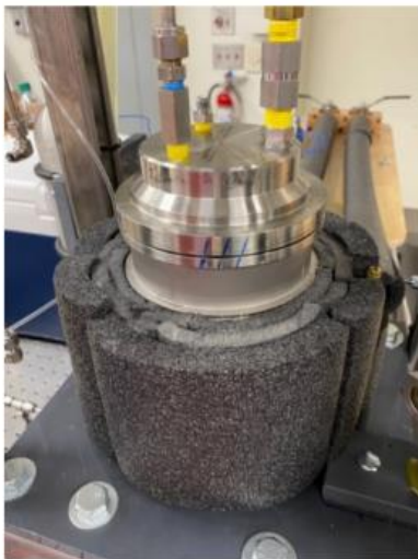
Figure 37: Vessel After Rings have been removed
