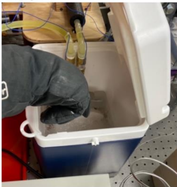
Figure 32: Adding Dry Ice to Auxiliary Chiller
