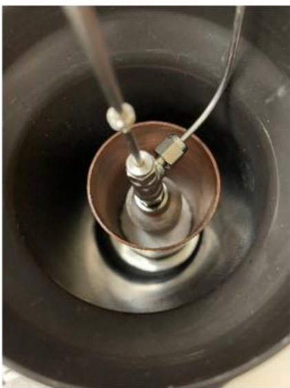
Figure 45: sample vessel inside the copper tube
