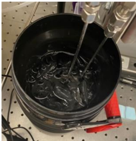
Figure 16: Heat Exchanger for Methane Gas
