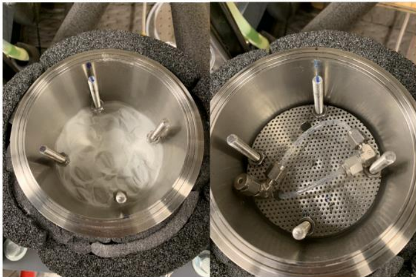
Figure 15. Basket with glass beads and perforated plate (lid) with halo water drip line
