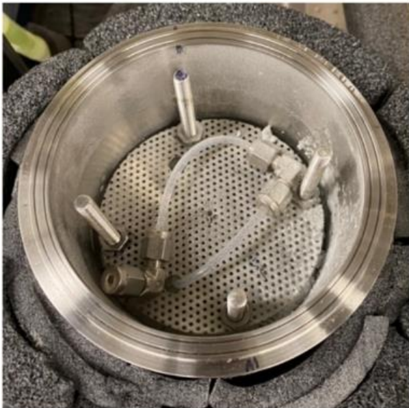
Figure 39: Wire Mesh is Lid of Basket. This should be removed
