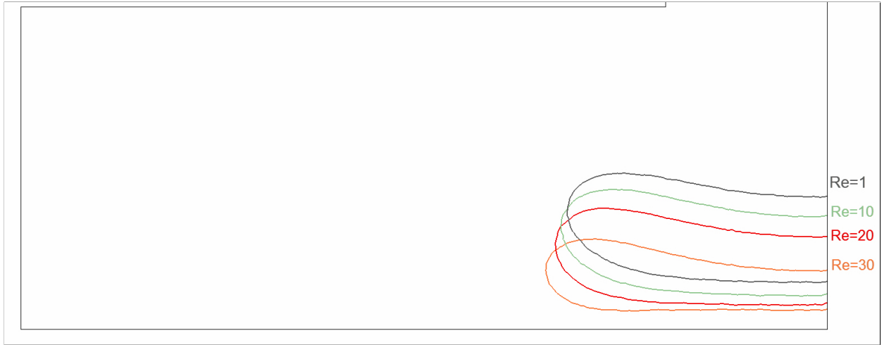
Figure 5.6: Bubble deformation. Neck thickness for different Reynolds numbers at the same non-dimensional time \tau .
