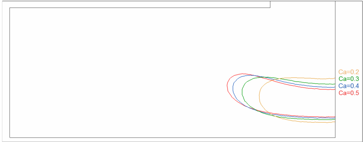
Figure 5.17: Neck thickness for \tau = 2.3 for different Ca and Re=10
