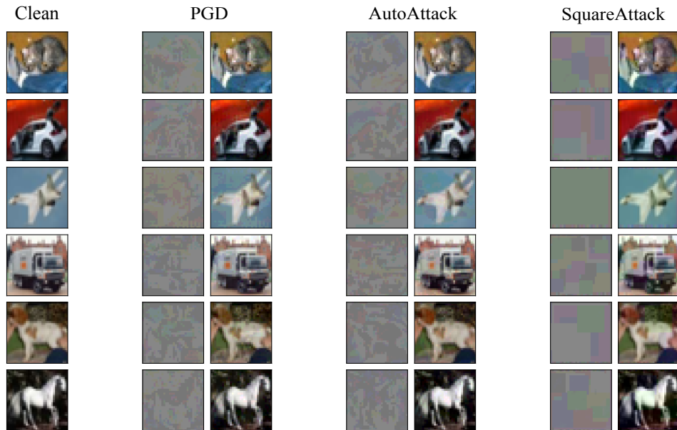
Figure 2.5: Illustration of three different attack types (PGD [9], AutoAttack [10], and SquareAttack [11]) and the corresponding perturbed images. Attacked images are not easily recognized by humans.
