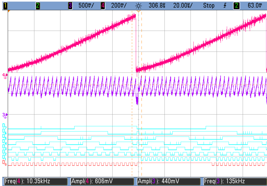
Figure 4.5: Oscilloscope recorded analog waveforms V_{IN} (red) and V_{OUT} (purple), and gray-coded digital ADC outputs (green) for (a) a linear ramp input, and (b) a sinusoidal input V_{IN} .
