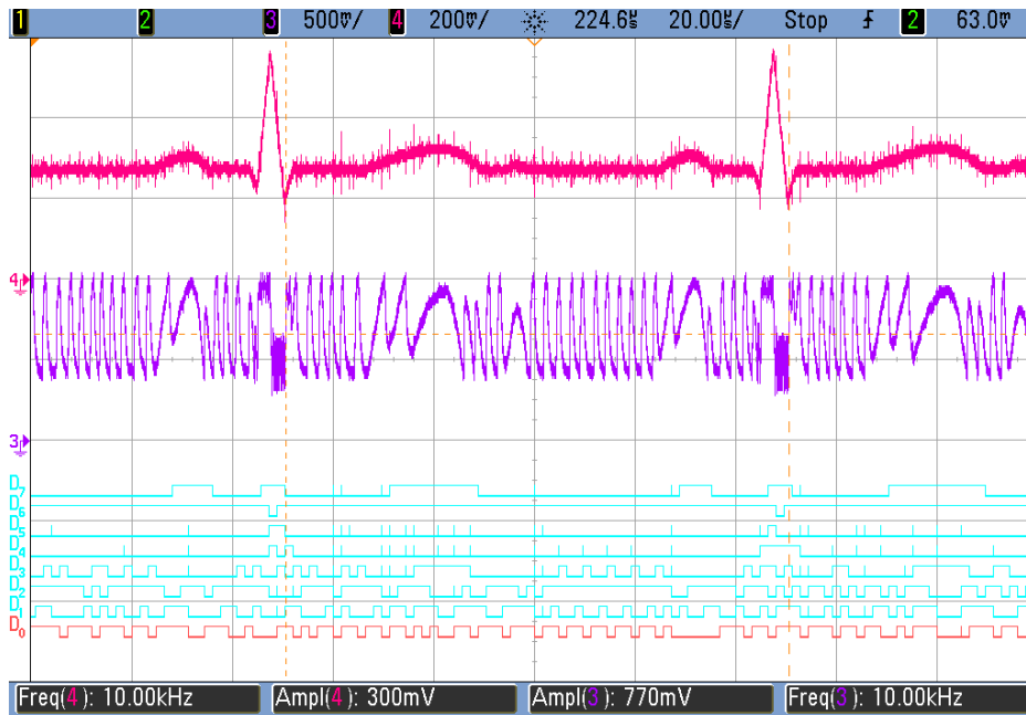
Figure 4.8: Sample ECG waveform recorded on oscilloscope: V_{IN} (red) and V_{OUT} (purple), and gray-coded digital ADC outputs (green).
