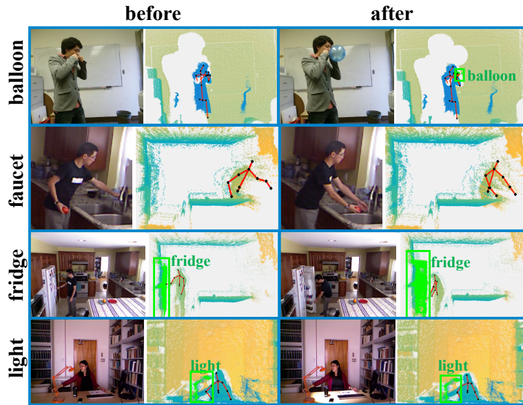
Figure 5.5: Human poses and depth images (before and after a fluent change) for actions as captured by the Kinect, together with sample frames.
