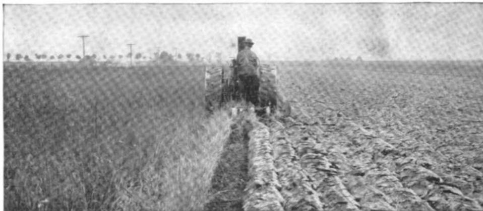
Plowing with an 8-16 Mogul in soil which was wet as well as mixed heavily with gumbo.
