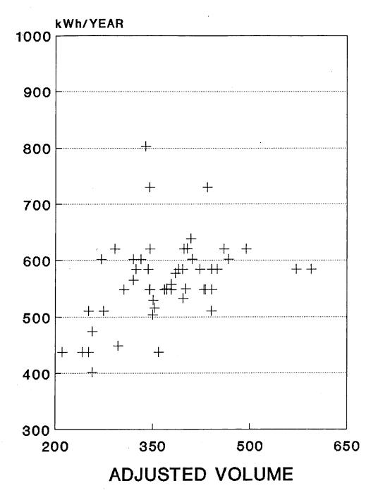
Adj. Vol.- refrig. vol.+1.8xfreezer vol Source: Mills 1989 from Konsumentverket
