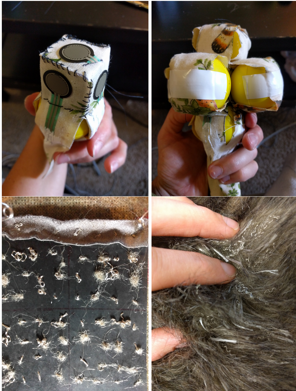
Figure 4.5: Construction of 6 degrees of freedom pressure sensor above. Conductive fur from below (left lower) and above (right lower).
