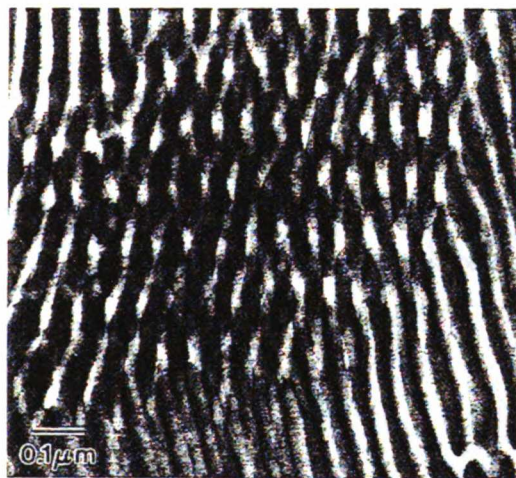
Figure 7. Conventional electron micrograph of an isolated region in the SI phase wherein (SI) 4 molecules have been trapped during macrophase separation. The presence of (SI) 4 molecules within SI lamellae serves to "pinch" the lamellae and consequently frustrate the local SI lamellar order, resulting in microdomain boundaries with nonzero mean curvature.
