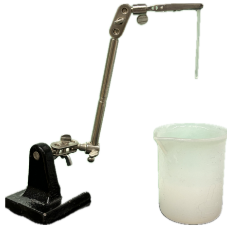
Figure 3.4. The mold setup for making the tubing
