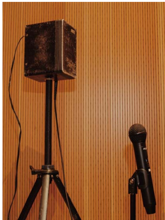
Figure 21: Non-optimal placement of “house” microphone (12 inch spacing) Photo Credit: H. Scott Roth
