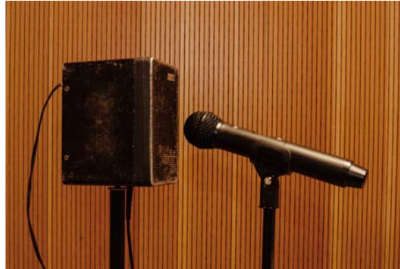
Figure 20: Optimal placement of “house” microphone (2 inch spacing) Photo Credit: H. Scott Roth
