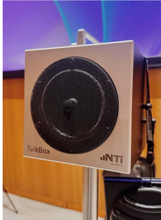
Figure 18: Nti Audio TalkBox used to measure STI Photo Credit: H. Scott Roth
