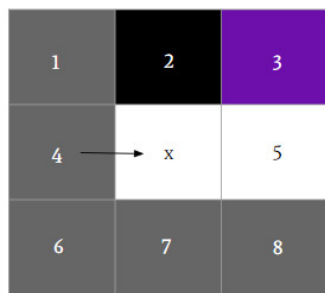
(a) Purple node No.3 is a forced neighbor of node x in a 2D map.
