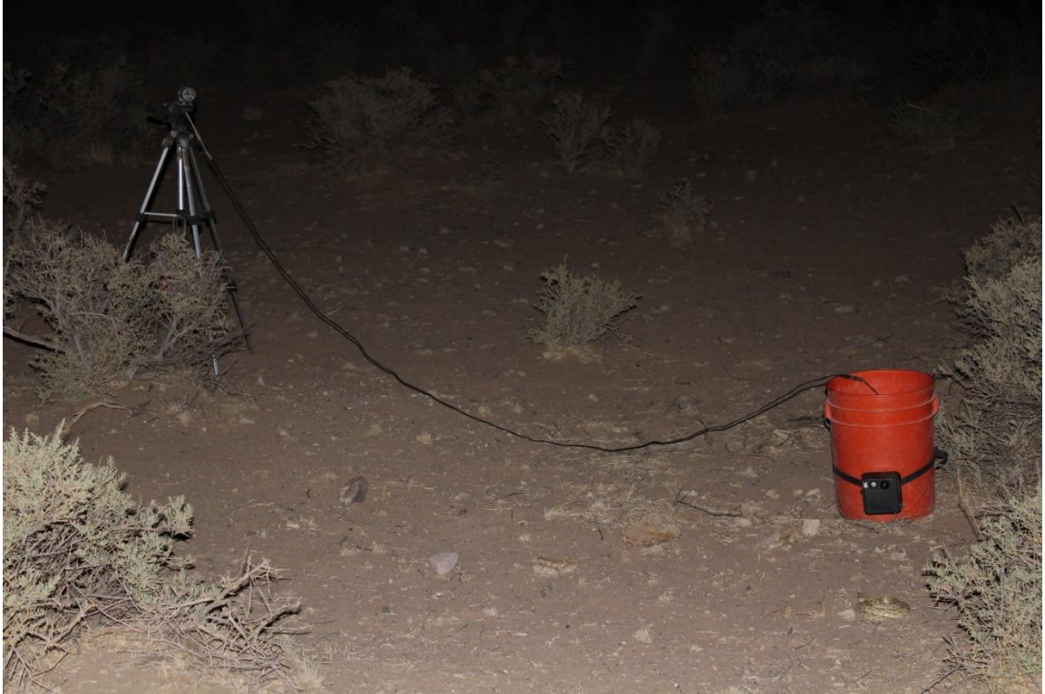
Figure 2.1: A typical example of the fixed-field videography unit used to study foraging ecology. The set-up consists of a near-infrared (IR) sensitive surveillance camera mounted 1 m from coiled snakes approximately 45° to the left or right side in front of the snake's head followed by a separate IR light positioned around 3 m away from the front of the snake to illuminate a 1 m 2 area around the snake. This unit is recording a Prairie Rattlesnake ( Crotalus viridis ), with the snake in the lower right corner of the photograph.
