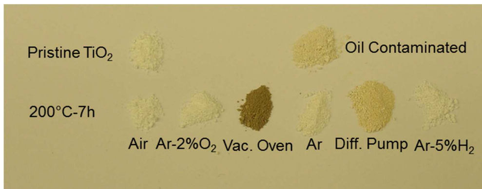
Figure 2.1 A photo comparing the color of TiO 2 powders annealed at 200 °C for 7 hours in different atmospheres as well as the pristine and “oil contaminated” TiO 2 .
