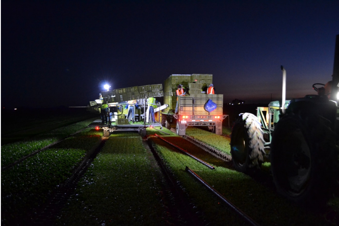
Figure 14. Factory line for packing baby greens on the move.
