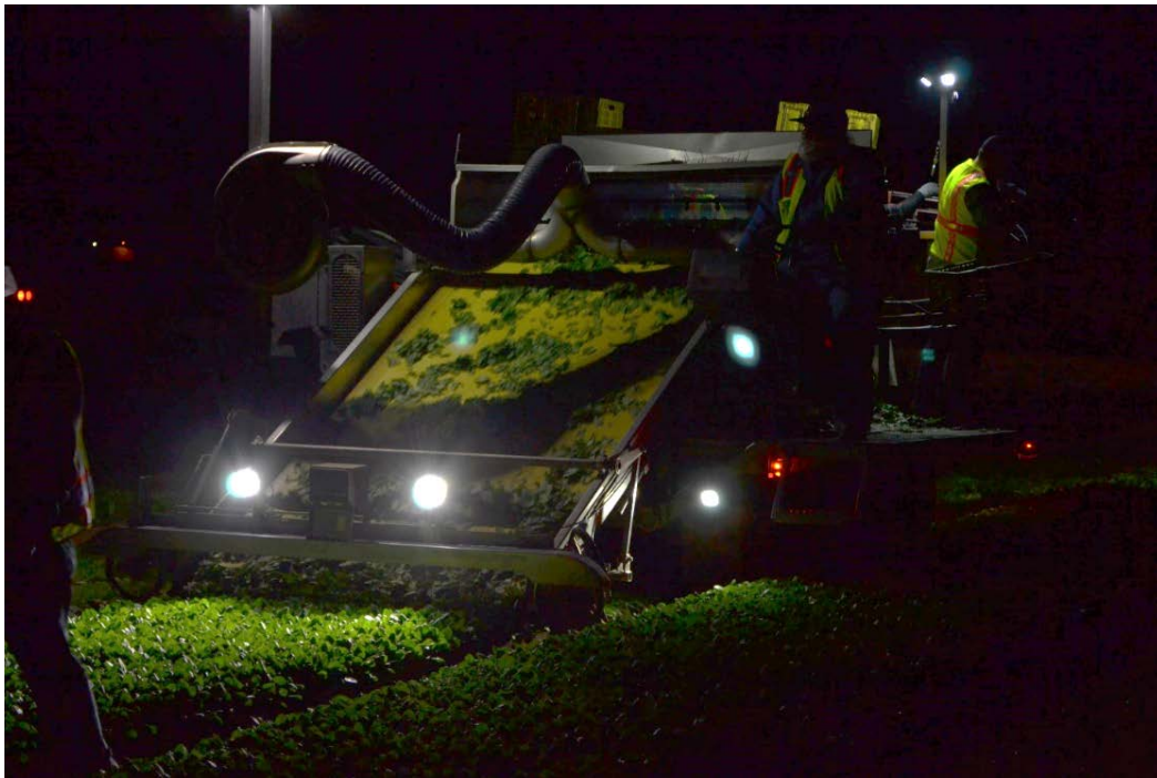
Figure 13. The harvest machine mowing baby spinach leaves.
