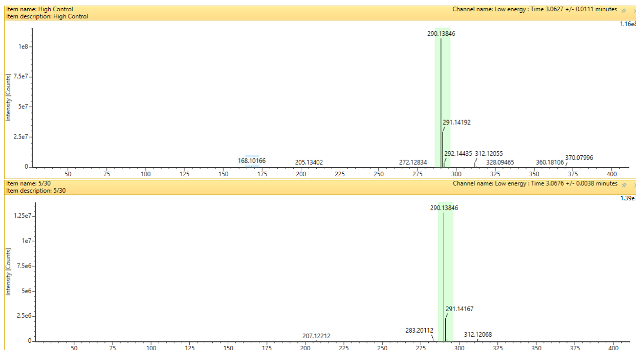
Figure A3. Low energy mass spectra for high control and sample 5/30 at approximately 3.06 minutes.
