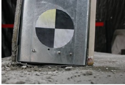
Figure 8.4: Photo showing rotation of connection similar to rotation observed in LS-DYNA simulation
