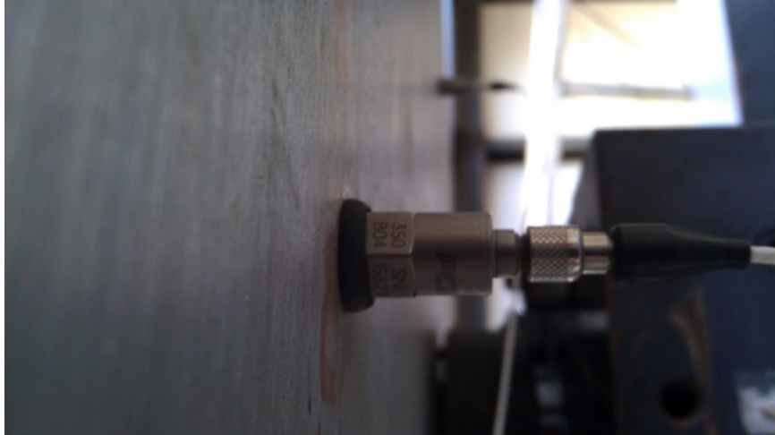
Figure 8.1: Rubber washer placed at interface between accelerometer and aluminum mass
