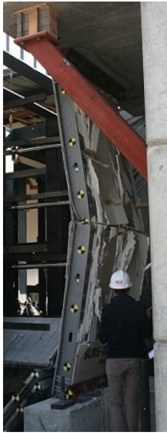
Figure 6.43: Test SSRE010-03.3 Damage
