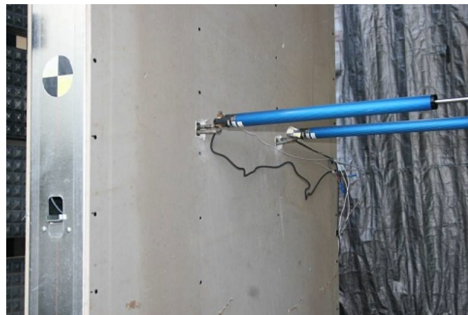
Figure 6.15: Detailed view of specimen accelerometers and LVDTs
