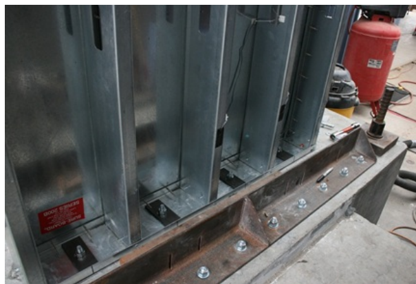
Figure 6.18: Test SSRE010-01 Lower Connection
