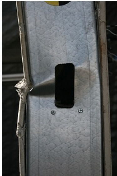
Figure 6.22: Test SSRE010-01 Primary Damage
