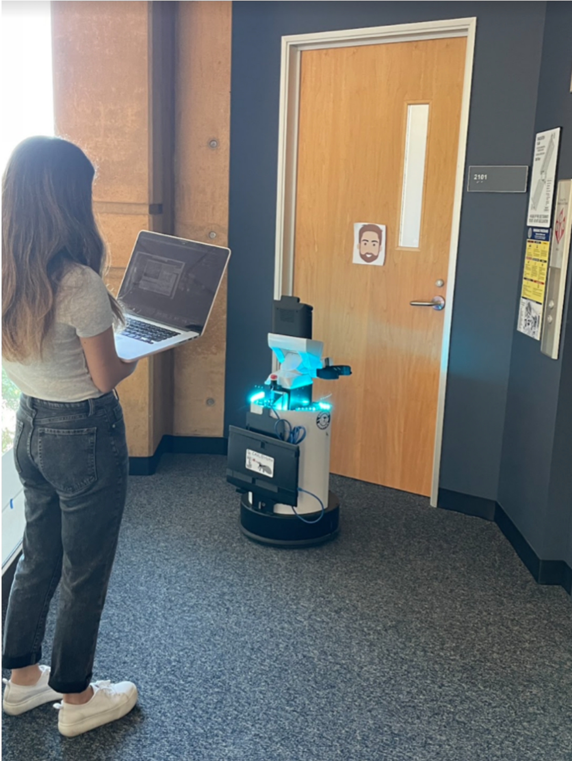
Figure 3.2: Participants were instructed to bring the cartoon face close enough to the camera to see the features of the face. The space of the robot to the face on the door represents the desired distance for each face. The experimenter followed behind the Toyota-HSR during the experimental sessions to check that the robot would not crash into any walls or obstacles.
