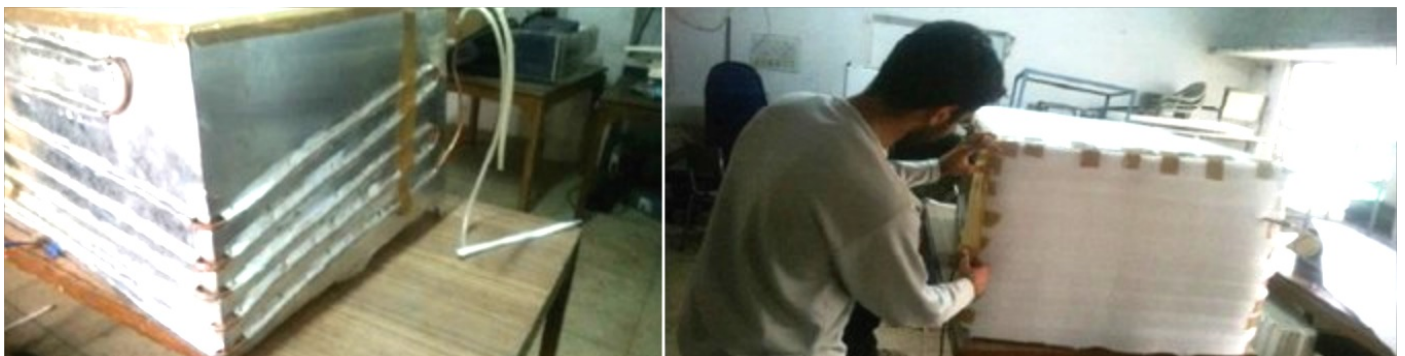
Figure 18: An experimental radiant cooling table for personalised cooling.
