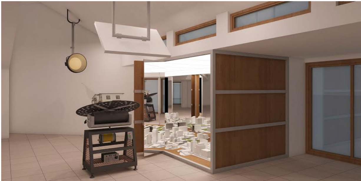
Figure 13: Artificial Clear Sky and Mirror Box
