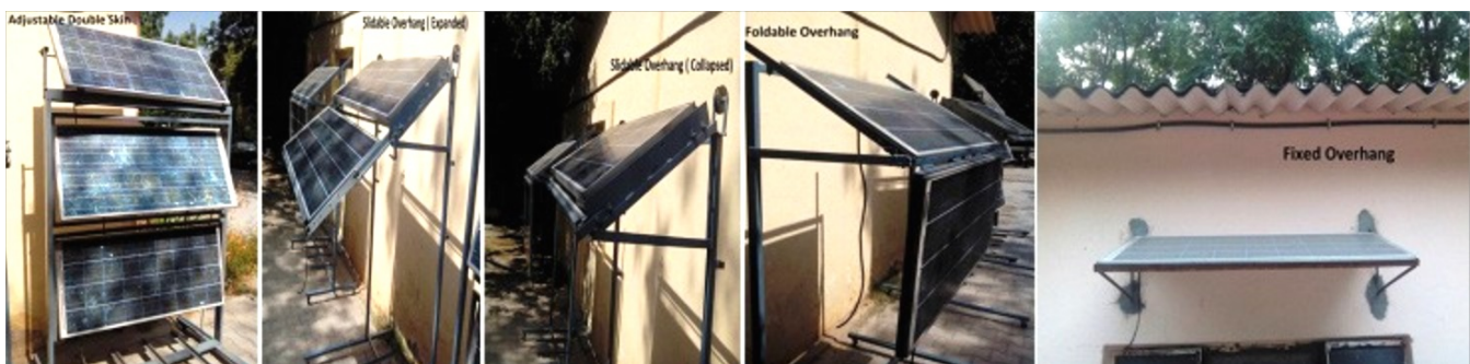
Figure 20: A BIPV prototype developed and being monitored
