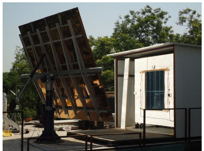
Figure 12: Testing of window with daylighting system for Solar Heat Gain Coefficient
