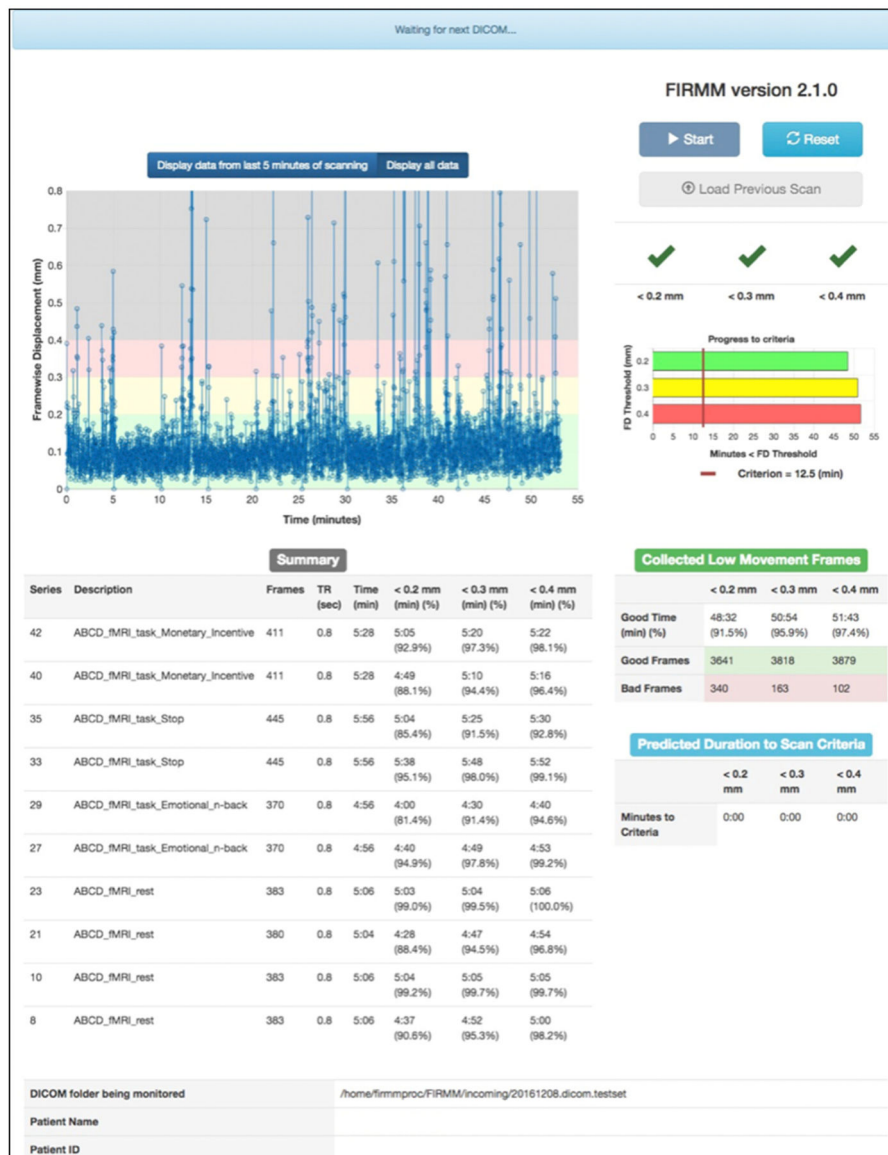
Fig. 1. Frame-wise Integrated Real-time MRI Monitoring (FIRMM) graphical user interface. Sample data are from the Adolescent Brain Cognitive Development (ABCD) study and include both task fMRI and resting state runs.
