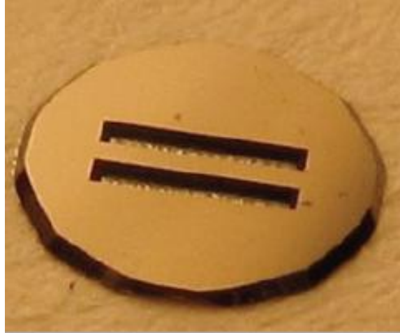
Figure 3.5. Grids for tomography. 5nm thick Si membrane is supported on a 100- \mu\text{m} -thick Si frame.
