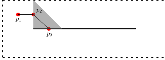
Figure 3.6: The thick line in the middle is the plate. \Gamma is the domain enclosed between the plate and the dashed rectangle (the spanwise direction is not visible in this figure). The shaded triangular region is R_T as defined in (3.70). Here, p_1 , p_2 , and p_3 are the points (x_1, x_2, x_3) , (0, x_2, x_3) , and (x_2, 0, x_3) . The point p_1 belongs to R_1 .
