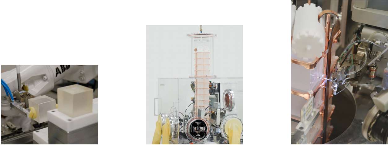
Figure 3.12: The CUORE assembly line. Left: The gluing robot attaches the NTDs and Joule heaters to the crystals under constant N_2 flux. Middle: All construction takes place in specially designed glove boxes under N_2 flux. The tower is stored in a garage immediately below the construction plane. Right: Wire bonding is done in situ with a specially mounted wire bonder.
